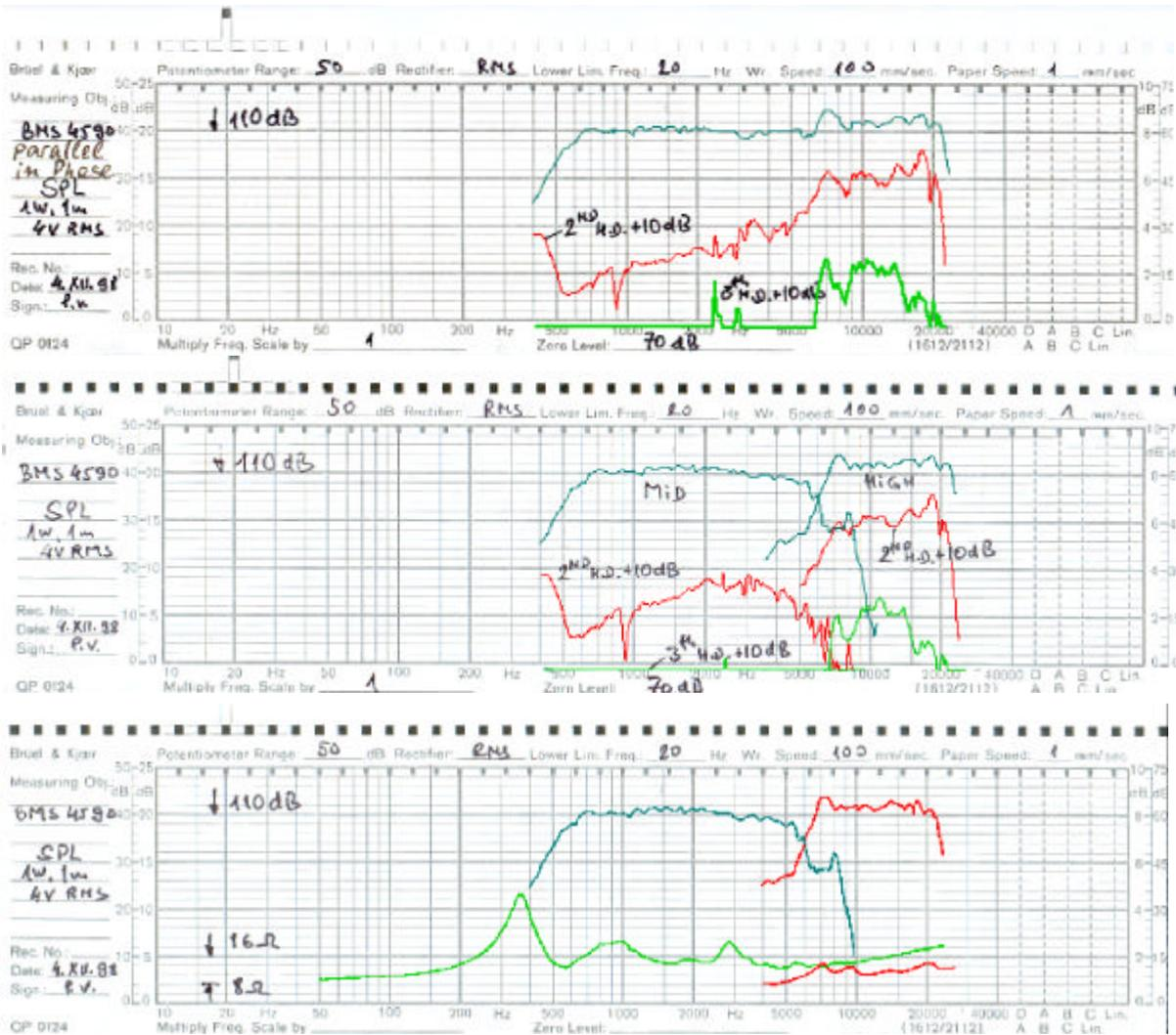
The driver is in fact a two way system employing two concentric annular ring diaphragms. The larger of the two reproduces middle frequency from 300 Hz upwards, crossing over over 6.3 kHz to the HF transducer which is capable of reaching 22 kHz. The voice coils may be driven together in conjunction with a passive crossover or driven individually from an active crossover.
